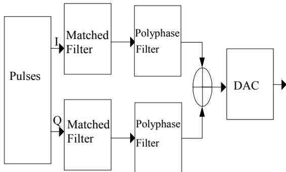
Figure 4 Digital modulator with interpolation
