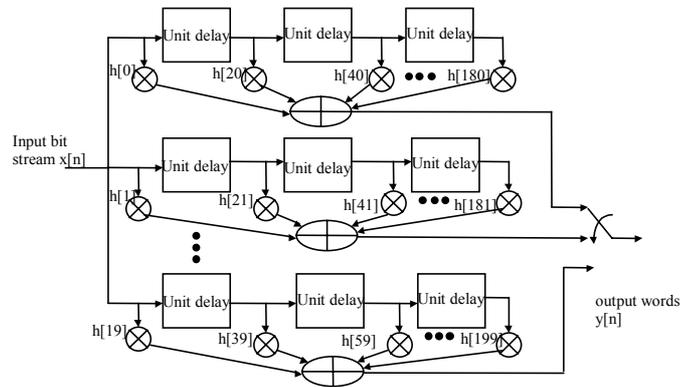
Figure 5 Polyphase implementation of 200 taps FIR filter
