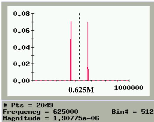
Figure 8 The spectrum of the signal after digitized at 2.5MHz. The alias frequency is 0.625MHz
