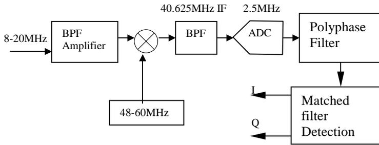
**Figure 2. Block diagram of the IF under sampling with Polyphase filtering method**
