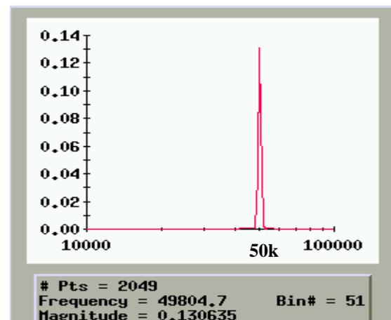
Figure 7 The output spectrum of the direct conversion method
