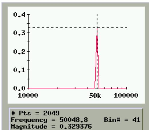
Figure 9 The output spectrum of the IF under sampling method
