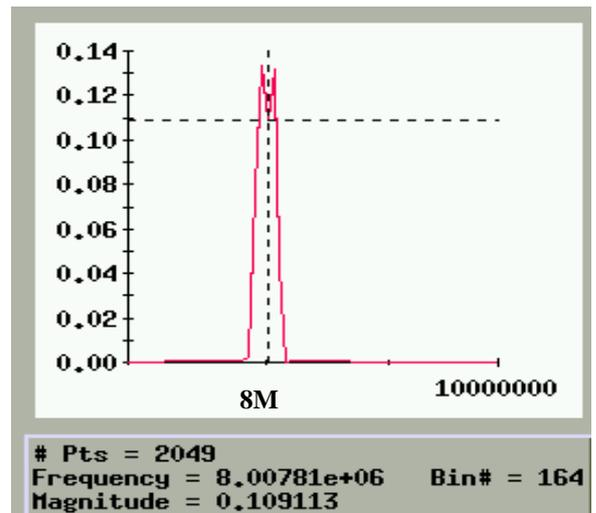
Figure 6 The spectrum of the modulated signal 8MHz, 100KHz bandwidth
