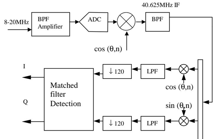
**Figure 4. Block diagram of the RF sampling method**
