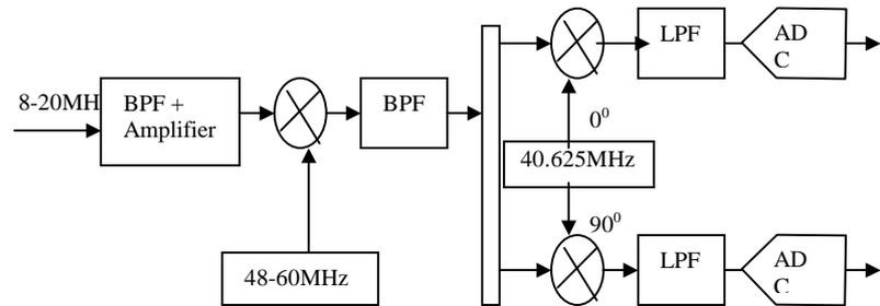
Figure 1. Block diagram of the base band digital techniques
