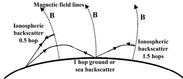
Fig. 5. Schematic ray paths showing 0.5 and 1.5 hop ionospheric scatter and one hop ground or sea scatter.
