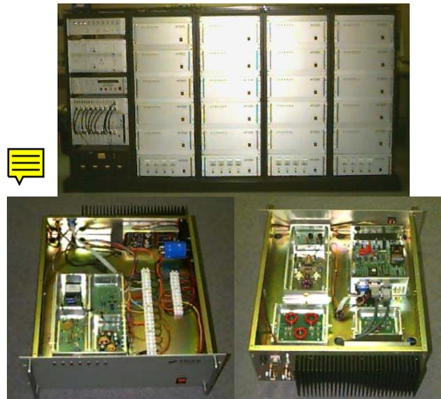
Fig. 3. TIGER Hardware. Top panel is a view of the front of the radar racks showing, on the right, the 20 transmitter modules above 4 power supplies. The receivers and phasing matrix are on the left. The bottom panels show views of a transmitter module chassis from the top (left) and bottom (right).
