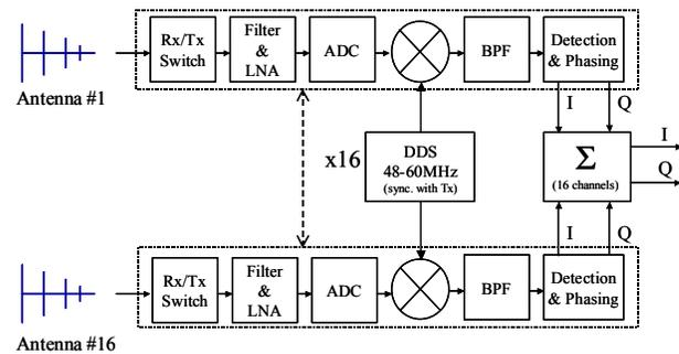
Fig. 11. Block diagram for proposed digital SuperDARN radar receiver even lower latitudes.
