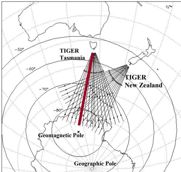
Fig. 1. Field of view of the TIGER radar. The straight lines represent the 16 azimuthal directions scanned by the  $\sim 3^\circ$  azimuthal beam of each radar. Beam 4 of the Tasmanian radar, (red) points along the geomagnetic meridian. The solid curved lines are contours of geomagnetic latitude and dotted lines contours of geographic latitude and longitude.
