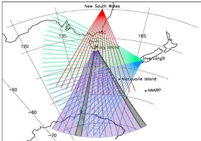
Fig. 9. Additional radars in NSW and NZ giving coverage to lower latitudes additional radars, one at Invercargill and one in NSW.
