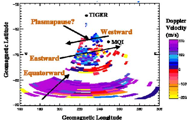
Fig. 7. TIGER scan showing scatter characteristic of several different ionospheric regions. Either another example should be used or this diagram improved to use the space better.
