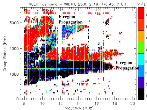
Fig. 6. Swept-frequency backscatter ionogram obtained along the magnetic meridian (beam 4). Echoes have been colour coded according to the Doppler spectral width and slow-speed, one-hop sea echoes are clearly differentiated from the high-speed 1.5-hop ionospheric scatter.
