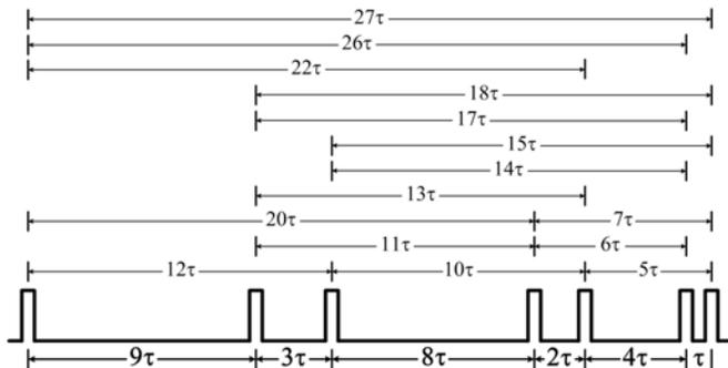
Fig. 4. SuperDARN Pulse sequence showing the various lags at which the autocorrelation function can be determined.
