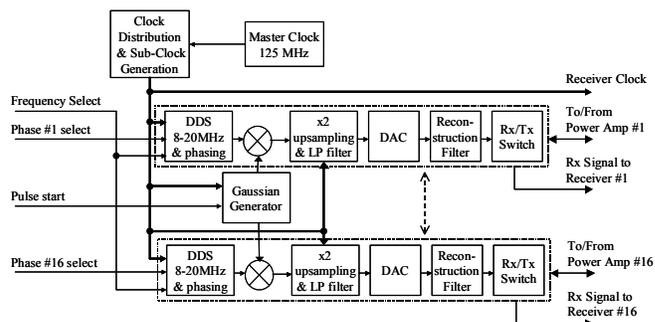
Fig. 10. Block diagram for proposed digital SuperDARN radar transmitter
